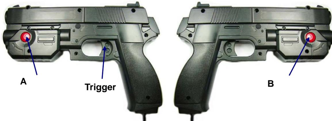
If you have bought the OEM electronics AimTrak kit then you will need to have wired up the Trigger, Aux and P1 connectors for the lightgun to work properly with Playstation 2.
