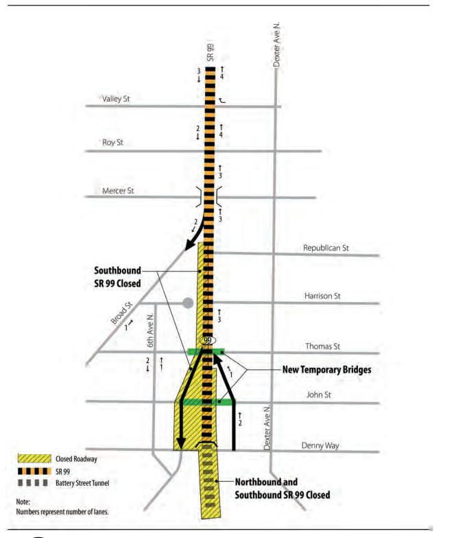
Exhibit 6-17 Cut-and-Cover Tunnel Alternative Traffic Stage 4 Roadway Configuration (North)
