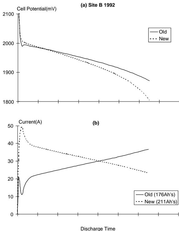
**Figure 5** 1992 Discharge Test for Site B, *Bank 1* (a) weakest cell behaviour and (b) sub-string discharge current.
