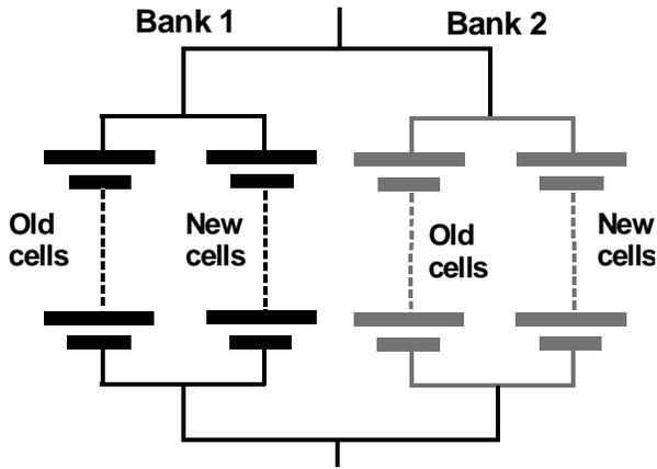
**Figure 4** Site B battery bank arrangement.
