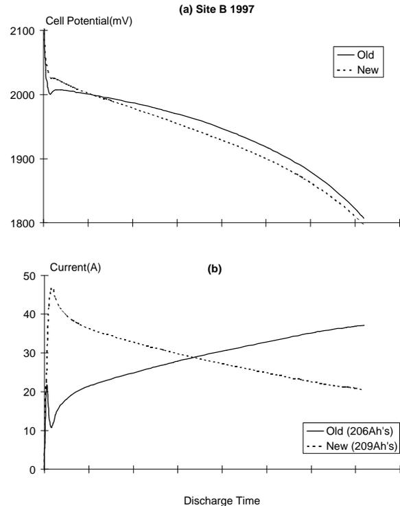
**Figure 6** 1997 Discharge Test for Site B, *Bank 1* (a) weakest cell behaviour and (b) sub-string discharge current.
