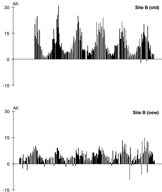
**Figure 7** Ampere-hour balances for Site B, Bank 1 “Old” & “New” sub-strings.
