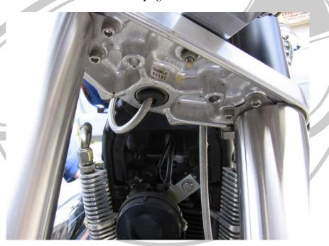
Use zip ties to secure the hose as needed to prevent chaffing or resting on a hot part of the engine.
