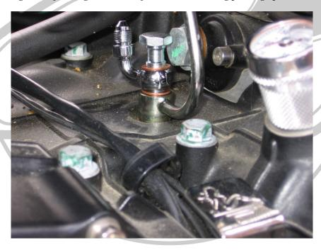
Thread the bolt with the 90 degree fitting through the oil feed line banjo and into the engine case then tighten to 20 N/M. \*\*DO NOT OVER TORQUE\*\* FAILURE TO FOLLOW TORQUE GUIDELINES CAN LEAD TO BOLT FAILURE AND CAUSE ENGINE DAMAGE.
