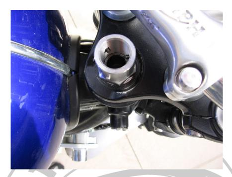
Insert the hose through the top of the neck and out the bottom.
