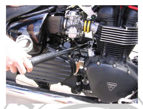
Route the hose rearward under the fuel tank, over the cylinder head and between the carbs down to the 90-degree banjo fitting.
