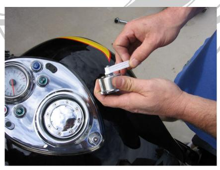
1 wrap only, do not cover the inlet hole of the gauge with the tape.
